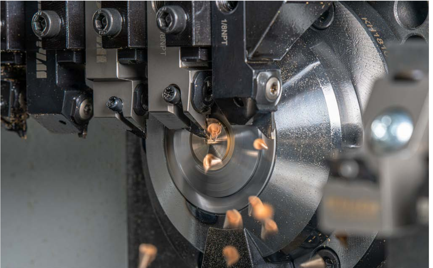
Turning high depth of cut, 8 mm, with the signature product range WhizCut. Resulting in great chip control and excellent surface finish.
